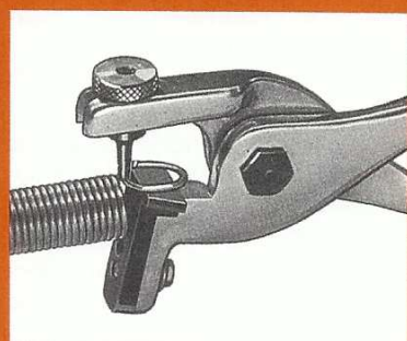
Fig. 8 Side loop in finished position.
