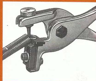
Fig. 6 Almost completed loop.
