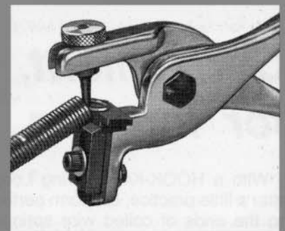
Fig. 6 Almost completed loop.
