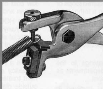
Fig. 7 Center loop in finished position.
